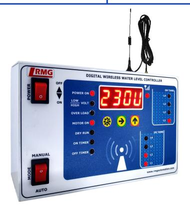
Wireless Fully automatic water level controller switches ON the motor when the water level in the tank becomes low (desired prefixed lower limit) making sure that water is present in the sump. It switches OFF the motor once the tank becomes full (prefixed higher limit) and also when the sump is empty.
