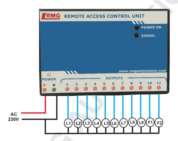
Figure 1: Power & Load connection
